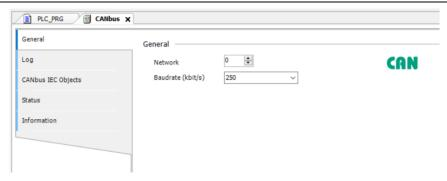
Figure 3-7 Parameter configuration of CANbus
