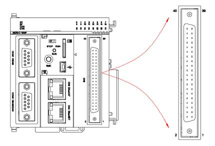
Figure 5.4 High-speed I/O wiring of the CPU module
