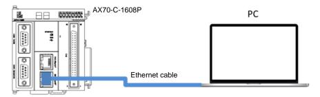
Figure 5.11 Ethernet connection
