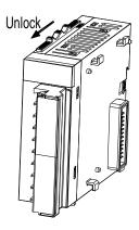
Step 2 Align with the connector on the CPU module for interlocking.
