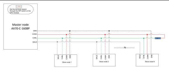
Figure 5.9 CAN bus connection
