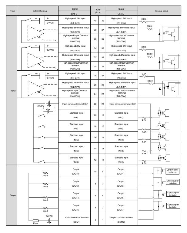
Figure 5.5 External wiring of high-speed I/O
