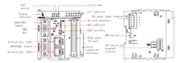
Figure 3.1 External interfaces of the CPU module
