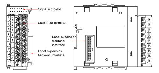
Figure 3.3 External interfaces of the digital input module
