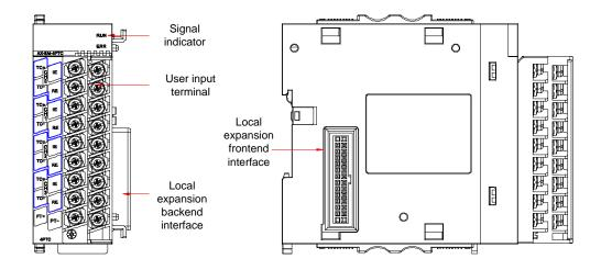
Figure 3.7 External interfaces of the temperature module
