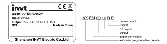
Figure 2.6 Digital output module
