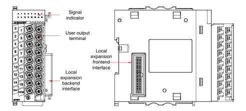
Figure 3.4 External interfaces of the digital output module
