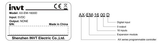
Figure 2.5 Digital input module
