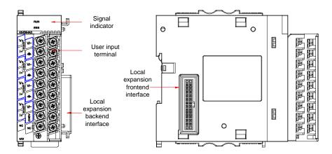
Figure 3.5 External interfaces of the analog input module
