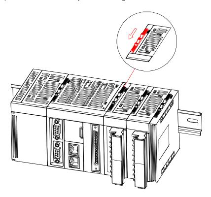
Slide the snap-fit on a module in the upward direction for unlocking.
