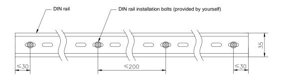
Figure 4.2 DIN rail installation (unit: mm)
