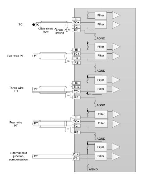
Figure 5.18 Terminal wiring
