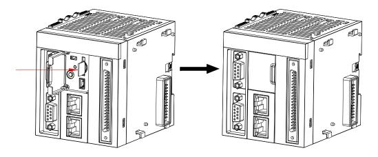
Figure 4.6 SD storage card disassembly
