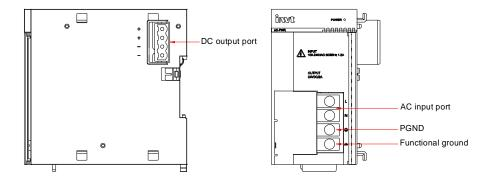
Figure 3.2 External interfaces of the power supply module
