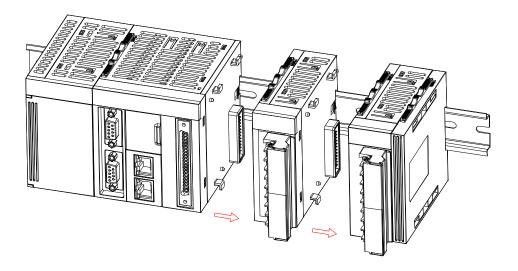
Slide the module in the arrow direction.
