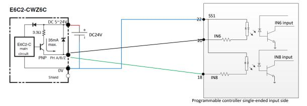
The preceding figure shows that phases A and B of the encoder whose output interface type is PNP are respectively output to CH6 and CH8 of the programmable controller.
