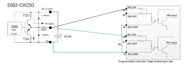
The preceding figure shows that phases A and B of the encoder whose output interface type is push-pull are respectively output to CH0 and CH1 of the programmable controller.
