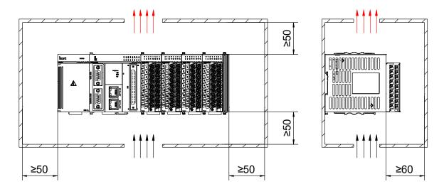
Figure 4.1 Requirements on installation space (unit: mm)
