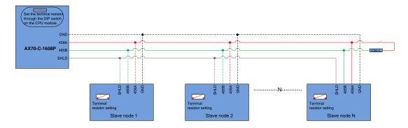
Figure 5.8 RS485 bus connection topology structure
