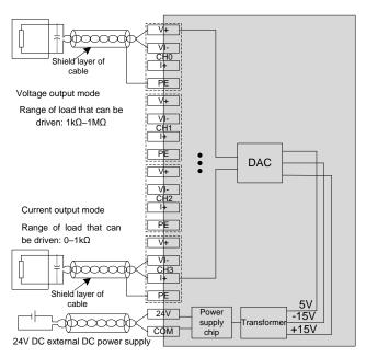
Figure 5.17 Terminal wiring
