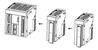
Step 3 Slide the snap-fit on analog input module in the direction shown in the following figure to connect and lock the two modules.
