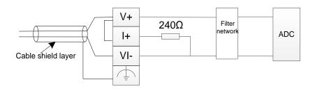
Figure 5.16 Wiring of current input
