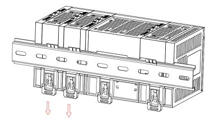
Pull the mounting hooks in the arrow direction.
