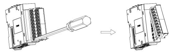
Figure 4.3 Terminal block disassembly
