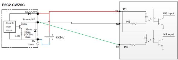
The preceding figure shows that phases A and B of the encoder whose output interface type is NPN are respectively output to CH6 and CH8 of the programmable controller.
