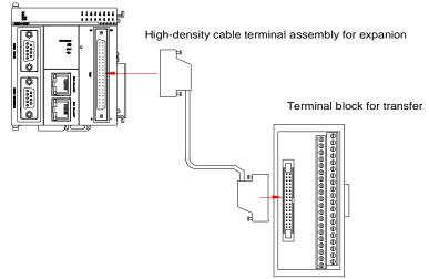
For connecting to HSIO signals on the user side
