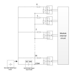
Figure 5.13 AX-EM-1600D terminal wiring
