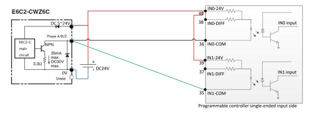
The preceding figure shows that phases A and B of the encoder whose output interface type is NPN are respectively output to CH0 and CH1 of the programmable controller.
