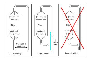
Figure 5.3 Power filter installation diagram
