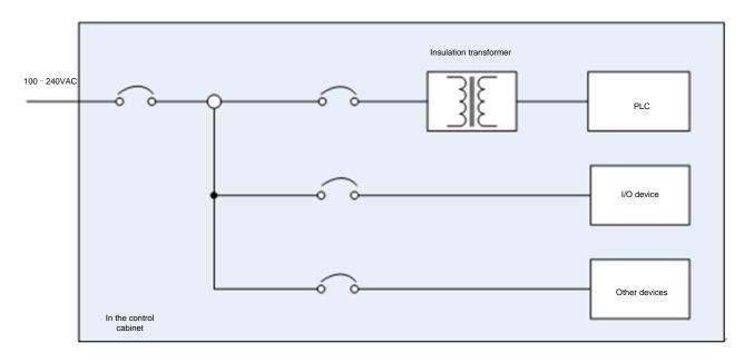
Figure 5.1 Insulation transformer working diagram
