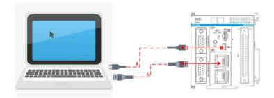
The hardware connection between an upper computer and programmable controller:
