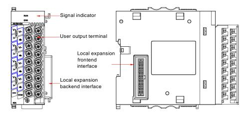
Figure 3.6 External interfaces of the analog output module
