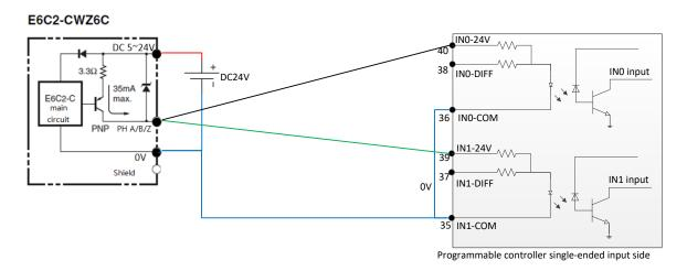
The preceding figure shows that phases A and B of the encoder whose output interface type is PNP are respectively output to CH0 and CH1 of the programmable controller.
