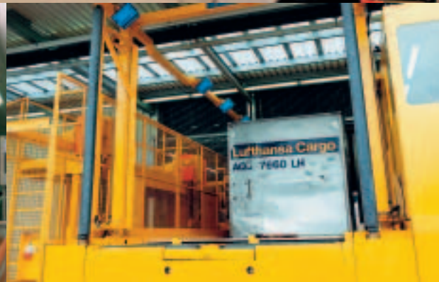
Volume measurement and checking for projections with the LMS: the system allows fully automatic loading of aircraft and prevents potential damage to aircraft projecting containers.
