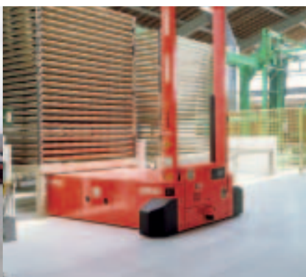
The LMS Laser Measurement System for preventing collisions outdoors on trucks without drivers.
