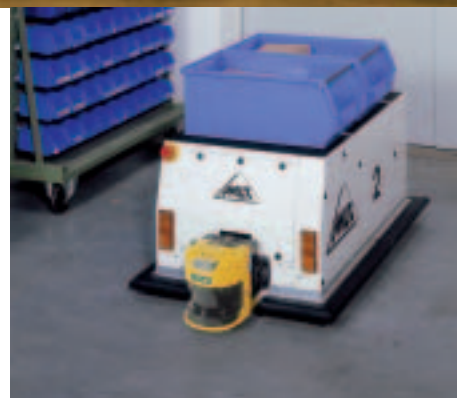
The S 3000 safety laser scanner is used here to protect a free-moving automated guided vehicle that transports small parts in boxes.
