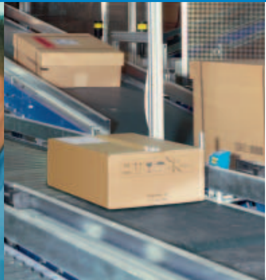
The WT 27 ASI photoelectric reflex switch determines the position of boxes on a roller conveyor system.
